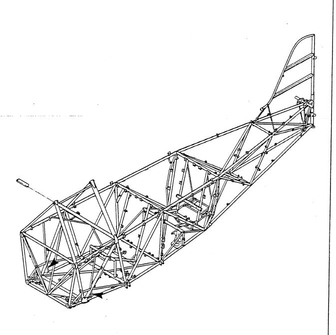
VERIFY THAT THE REINFORGMENT TUBES MARKED WITH AN ARROW HEAD ARE ATTACHED
