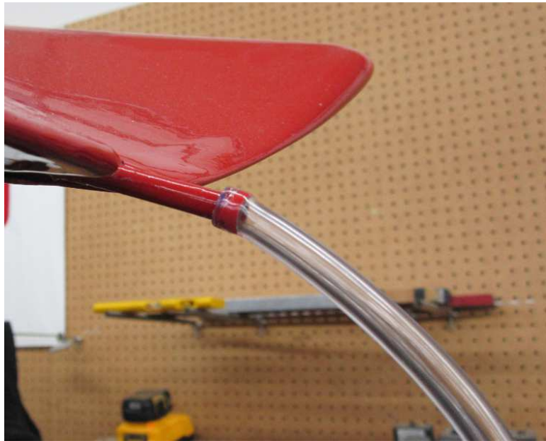
Figure 2. Supplied clear plastic test tube pushed onto the fuel vent line.
