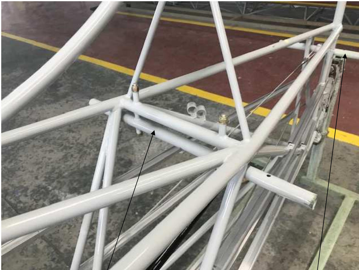
Figure 1, Stabilizer Support Assembly, fabric removed for clarity. Tube 30800-111
