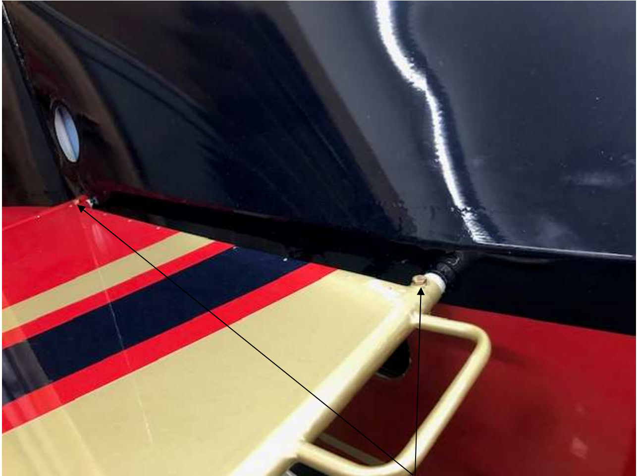
Figure 6, Tail fairings removed and AN3 attach bolts shown
