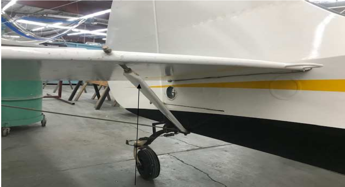
Figure 7, Stabilizer strut assembly
