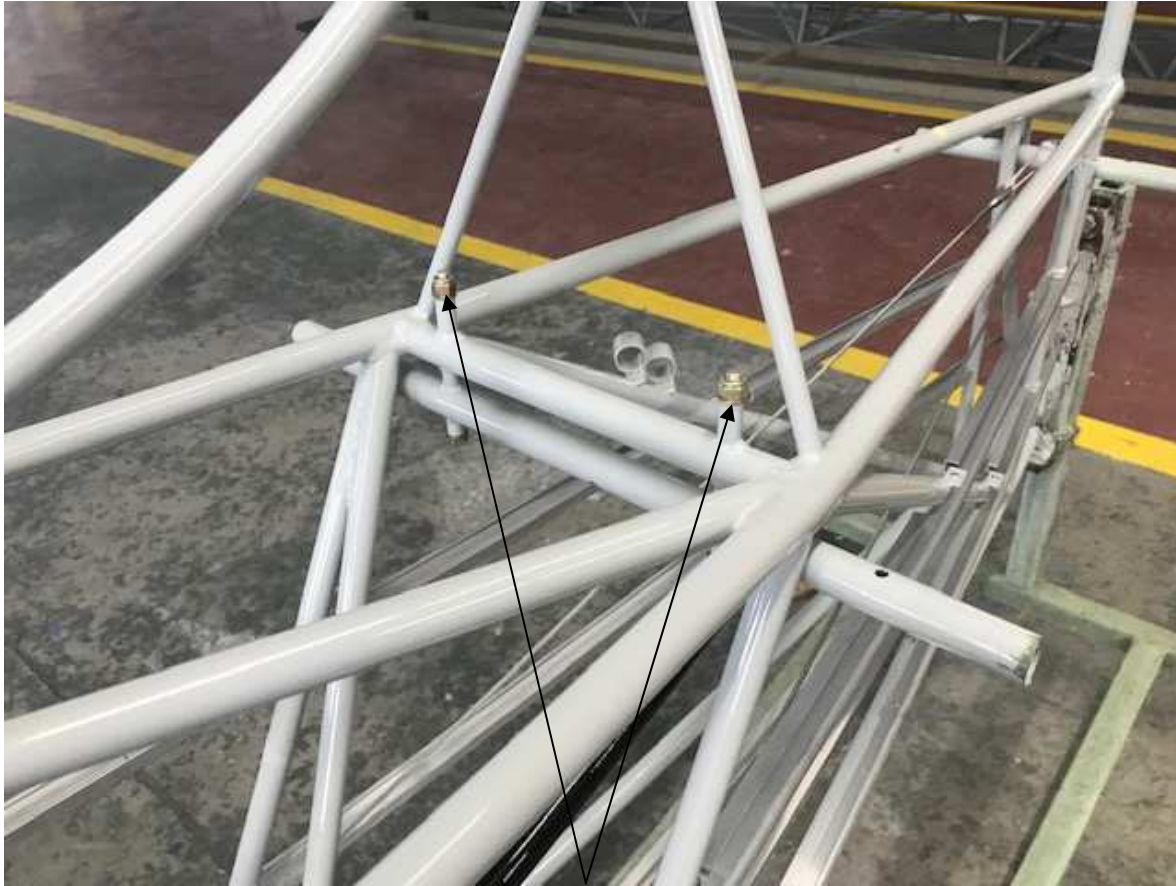
Figure 9, AN4 Bolts, fabric removed for clarity
