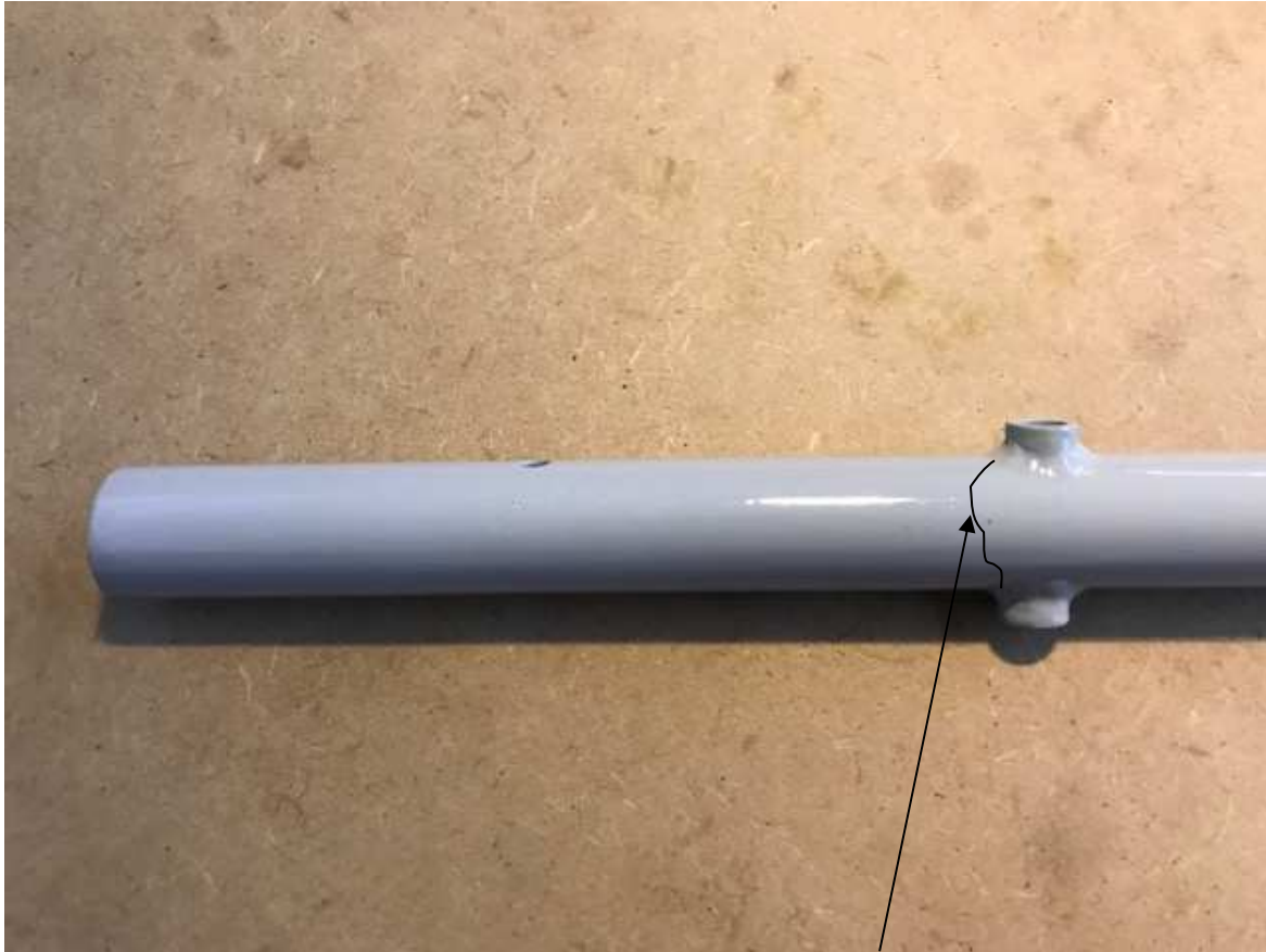
Figure 5, Typical crack location
