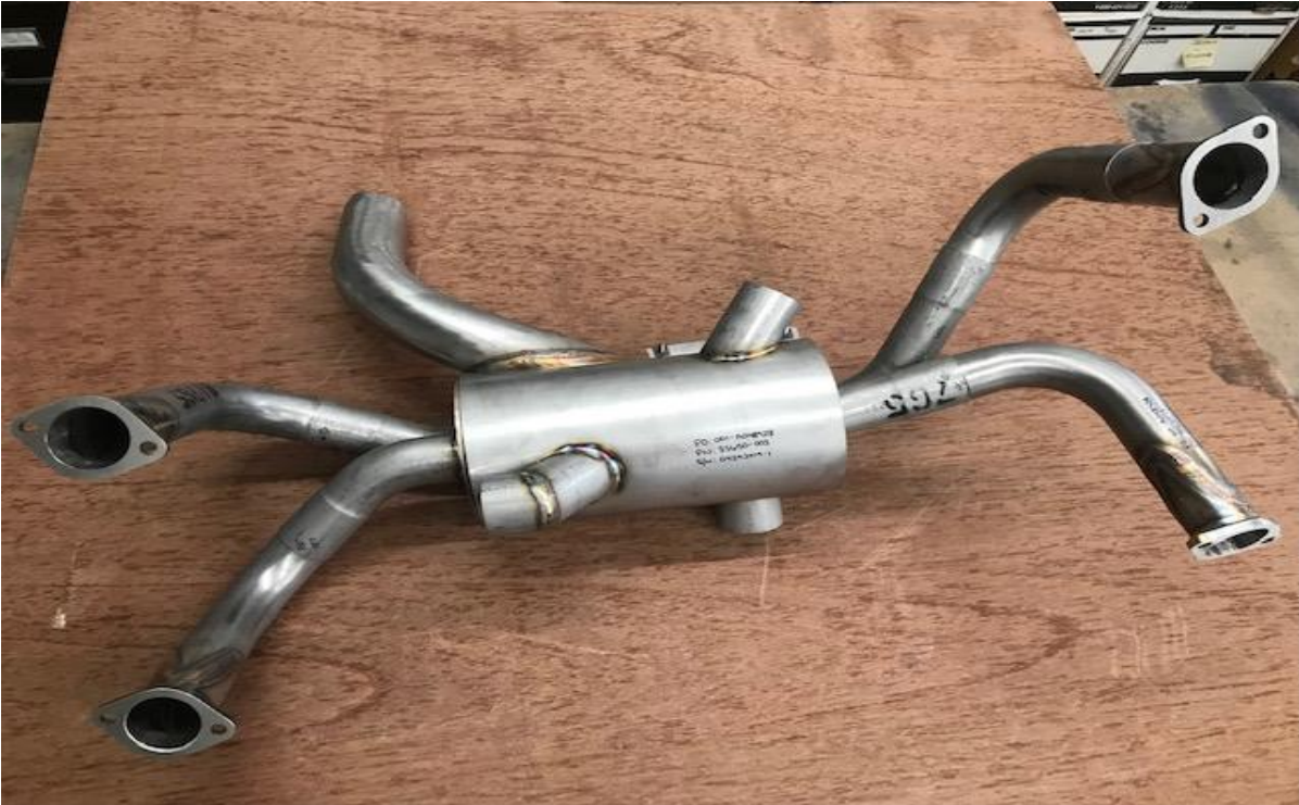
Figure 6: removed exhaust assembly
